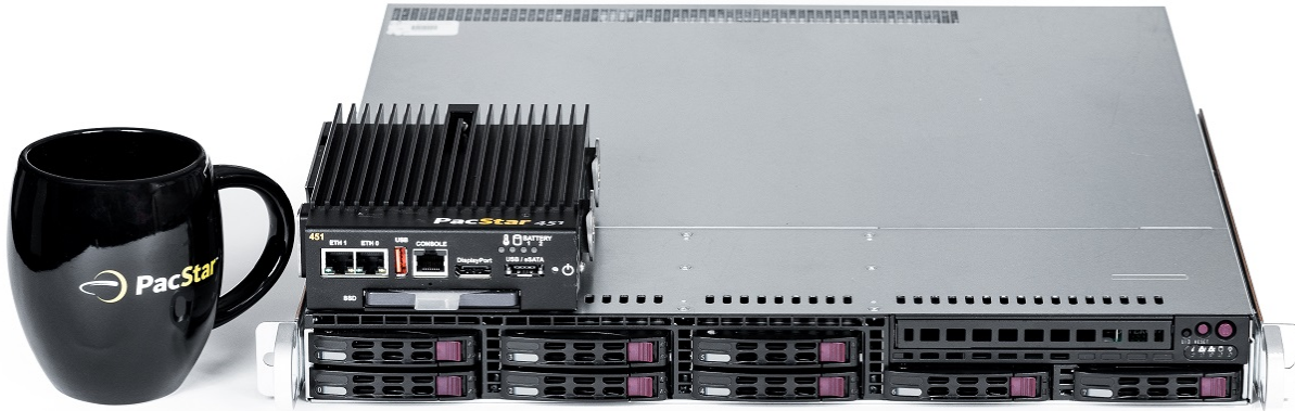
Figure 7: Illustration of SWaP savings from tactical equipment vs. 19” rack mount legacy gear
