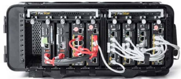
Figure 9: Modular, Tool-less, Dockable, Dismountable Chassis with Built-in UPS.[7]
