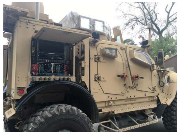
Figure 8: Rugged Communications Equipment Mounted on Marine Corp JLTV[6]
